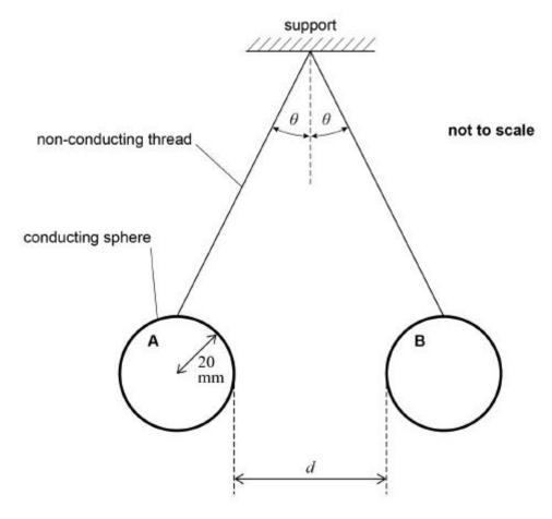
Each sphere has a mass of  $3.2 \times 10^{-3}$  kg and a radius of 20 mm. The distance d is 40 mm.
