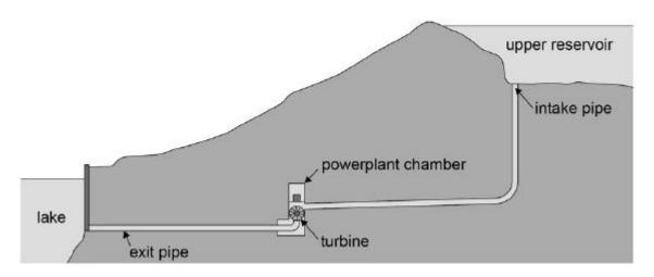
Water from the upper reservoir is to fall through a vertical distance of 90 m before reaching a powerplant chamber. The water rotates a turbine in the chamber that drives an electricity generator. After leaving the turbine, the water travels through an exit pipe to a lake.
