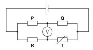
The temperature of the negative temperature coefficient thermistor **T** is then increased.
