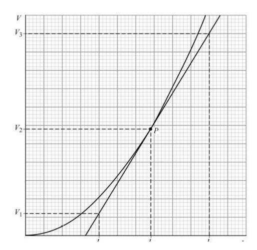
What is the resistance of the electrical component when the current in the component is  $I_2$ ?
