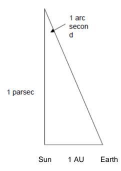
1 pc is the distance at which 1AU subtends an angle of 1 arc second
