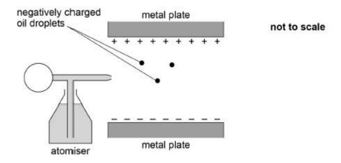
Negatively charged oil droplets are sprayed from the atomiser into the gap between the two horizontal metal plates. A potential difference is applied between the metal plates.
