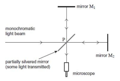
In the apparatus, light waves reflected by the mirrors  $M_{\scriptscriptstyle 1}$  and  $M_{\scriptscriptstyle 2}$ , meet at P so that they superpose and produce interference fringes. These are observed using the microscope.
