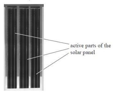
(i) By taking measurements from the full size photograph, show that the total area of the active parts of the solar panel is about  $10^{-3}$  m<sup>2</sup>. Include the uncertainty in your answer.
