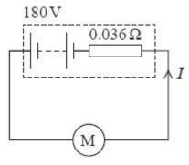
The motor has a maximum power of 88 kW.
