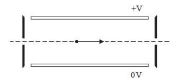
In one mass spectrometer the plates are 2.5 cm apart and a p.d. of 135 V is applied.
