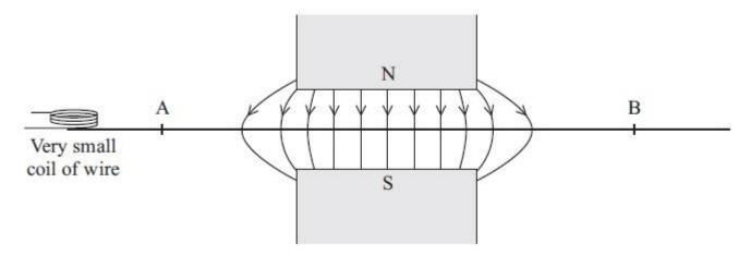
Sketch a graph to show how the e.m.f. induced across the coil varies as the coil moves from A to B at a constant speed.
