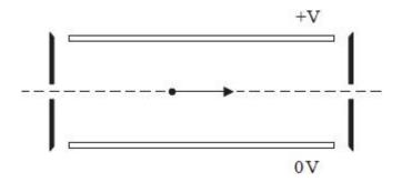
In one mass spectrometer the plates are 2.5 cm apart and a p.d. of 135 V is applied.
