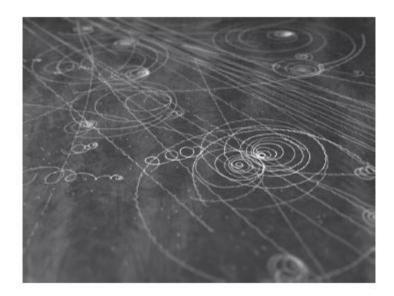
Modern particle detectors such as the ones at CERN still work on the basic principle that charged particles cause ionisation of the material through which they pass. These ionisations can be tracked and recorded. Magnetic fields are used to deflect the particles so that their properties can be investigated.
