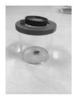
The lid has a built-in lens and an additional optional lens to allow the magnification to be increased.
