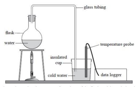
The water in the flask was heated and steam was forced out of the flask and through the glass tubing into the cold water in the insulated cup. The steam condensed as it passed into the cold water.
