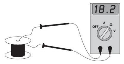
The diameter of the wire was measured as 0.27 mm  $\pm$  0.01 mm. The length of the wire was measured as 1.25 m  $\pm$  0.05 m.
