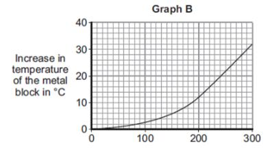
After 300 seconds, **Graph B** shows the increase in temperature of the metal block is lower than the increase in temperature expected from **Graph A**.
