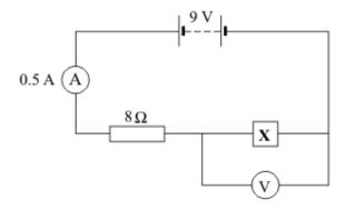
(i) Calculate the potential difference across the 8 ohm resistor.
