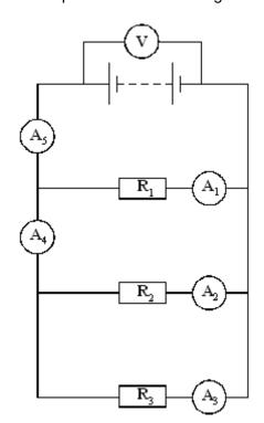
(a) The table gives the current through three of the ammeters. Complete the table to show the current through the other two ammeters.
