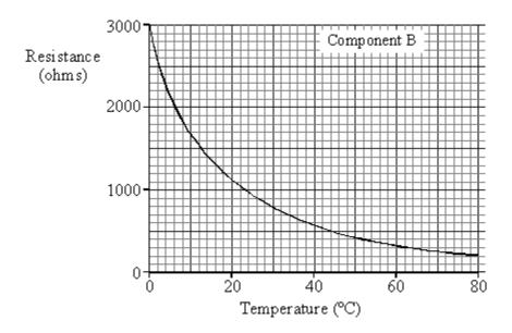
Describe, in as much detail as you can, how the resistance of component B changes as its temperature rises from  $0^{\circ}\text{C}$  to  $80^{\circ}\text{C}$ .
