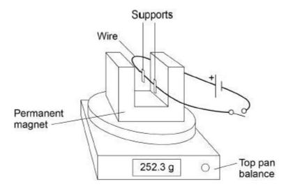
The top pan balance was used to determine the force on the wire.
