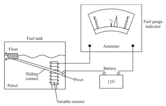
(a) Use standard symbols to draw a circuit diagram for the fuel gauge assembly.
