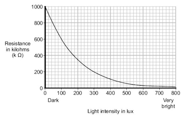
Describe how the resistance of the LDR changes when the light intensity increases from 100 lux to 300 lux.
