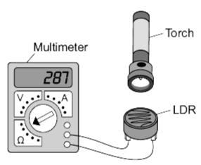
The resistance of the LDR was measured directly using a multimeter.
