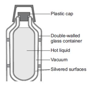
A vacuum flask is designed to reduce the rate of energy transfer by heating processes.
