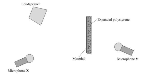
(ii) The student tests four materials. Each sheet of material is 1 mm thick. This has been glued onto a block of expanded polystyrene.
