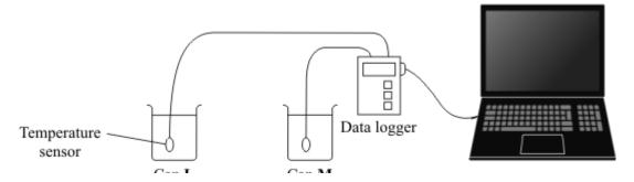
The student filled the two cans with equal volumes of hot water. He then placed the temperature sensors in the water and started the data logger. The computer used the data to draw the graph below.
